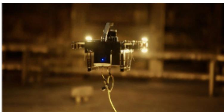
It is understood that the DNV-led project is testing drone technology, developed by Scout Drone Inspection that are capable of navigating in confined spaces, such as cargo tanks. This provides valuable input and requirements from the owner’s perspective for future drone tank surveys. DNV recently adapted their survey process for the use of drones and implemented supporting software.
